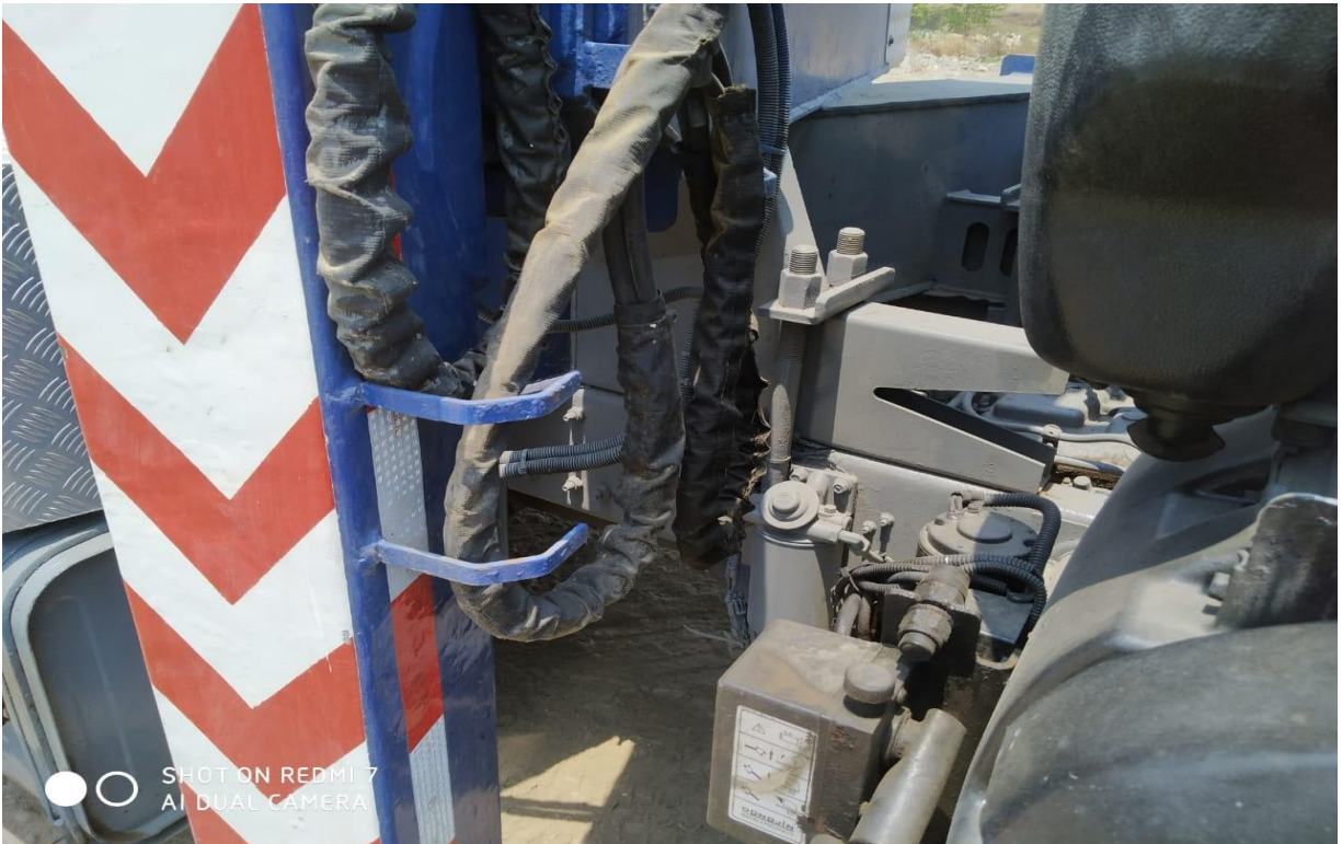
Picture-3 Bolting of chassis of vehicle and beam of Sky lift just behind the vehicle cabin
