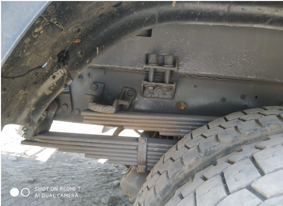
Picture-5 The bolting of the Skylift with the back side of the chassis
